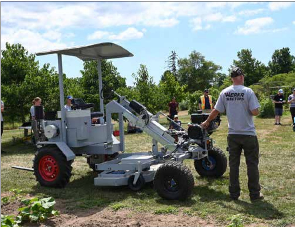
The Werkr electric tractor is a made-in-Canada solution for tractor automation. The company started with contracts from major lawn tractor manufacturers.
