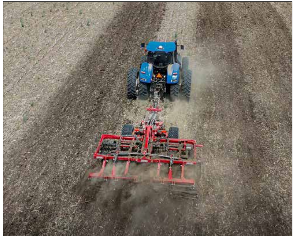
Salford Group Inc.'s fastest growing product is the HALO VRT, which "allows producers to adapt to soil and residue conditions by hydraulically changing their tillage intensity on-the-go," said Anson Boak, marketing manager for the company.
