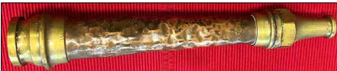
A smooth bore nozzle made of brass and copper.
