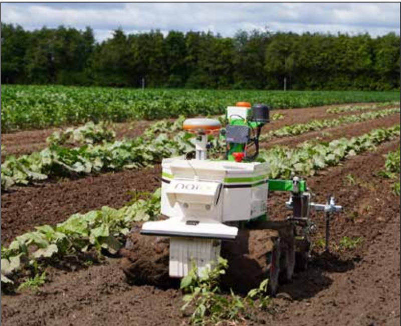
The NAIO Oz Robot works in a demonstration field, showcasing its ability to sow, mark rows, cultivate and weed in market gardens and specialty crops. The demonstration was part of Ag Robotics Demo Day, held July 22 at the Ontario Crops Research Centre in Simcoe, a University of Guelph research station. ~ Amanda Nelson photos
