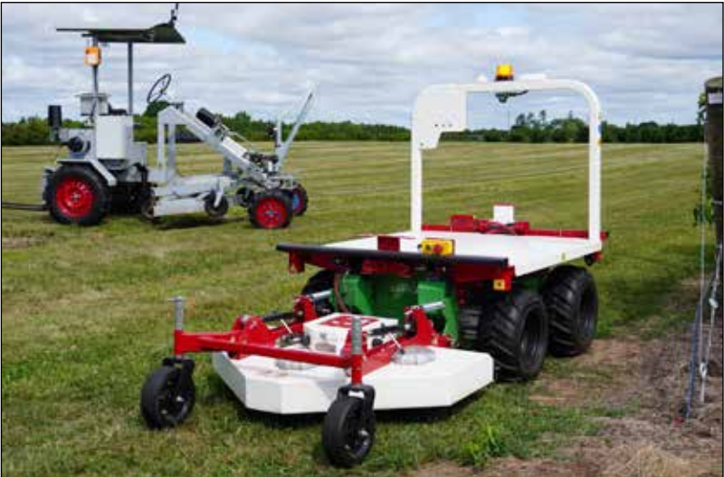
Burro Robotics demonstrates autonomous technology that uses computer vision, high-precision GPS and artificial intelligence to follow people and navigate independently while performing a range of agricultural tasks.
