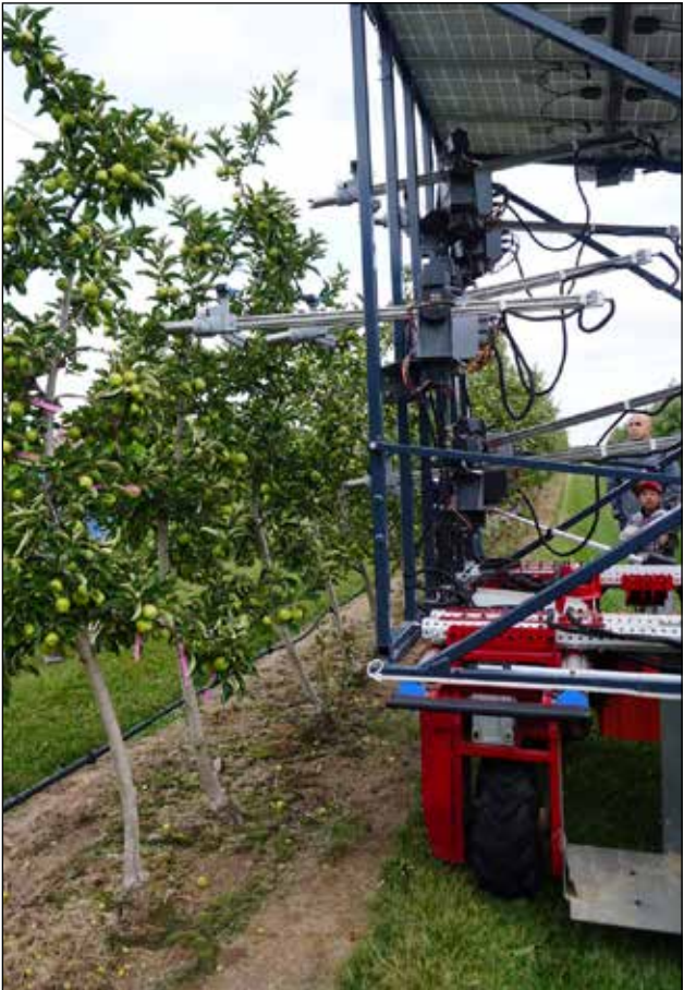
Finite Robotics demonstrates its fruit-thinning technology, designed to automate labour-intensive orchard tasks such as fruit counting, crop-load measurement, tree-health monitoring and yield estimation.
