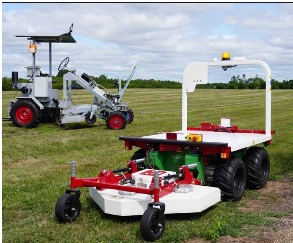
Burro Robotics demonstrates autonomous technology that uses computer vision, high-precision GPS and artificial intelligence to follow people and navigate independently while performing a range of agricultural tasks.
