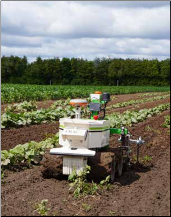
The NAO Oz Robot works in a demonstration field, showcasing its ability to sow, mark rows, cultivate and weed in market gardens and specialty crops. The demonstration was part of Ag Robotics Demo Day, held July 22 at the Ontario Crops Research Centre in Simcoe, a University of Guelph research station.
