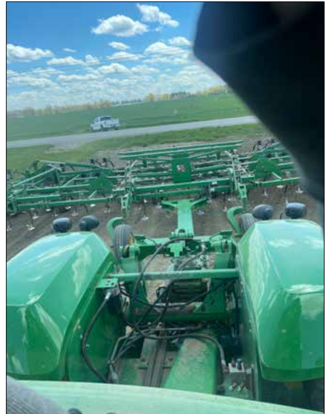
Looking back from the cab of Dave Meadows' John Deere 9330 tractor as the 50-foot cultivator works the field. Meadows says the operation can cultivate 25-30 acres per hour at about five miles per hour.
