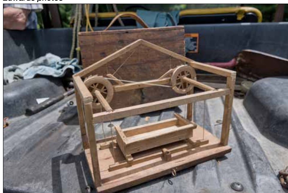
This model rack lifter would have been taken around to local farmers to show how the real thing could help them unload hay in their barns.
