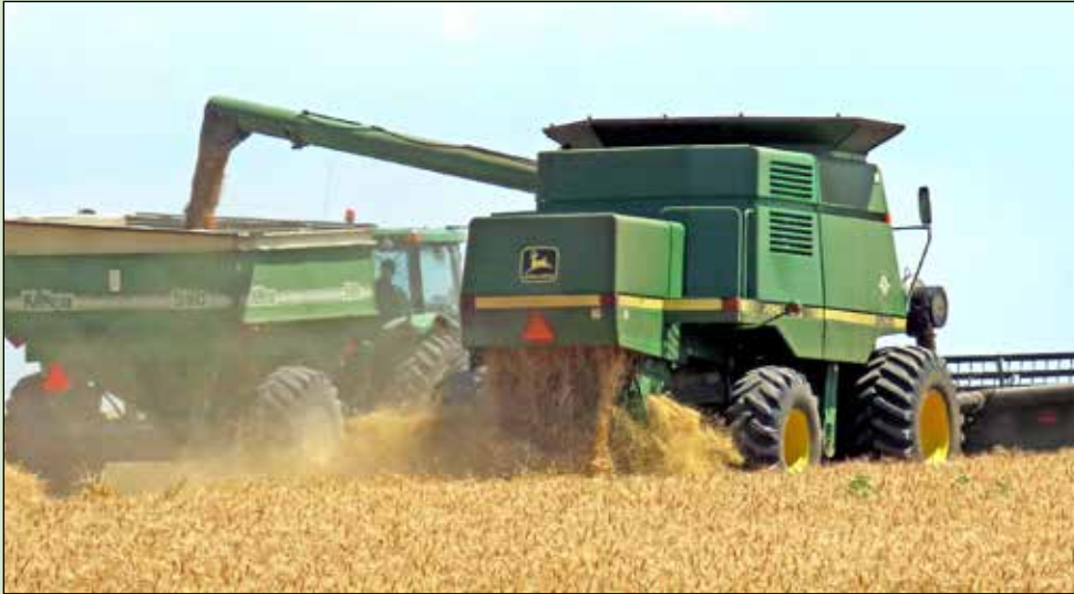
Combine with chase buggy alongside, emptying hopper/tank while continuing to harvest.
