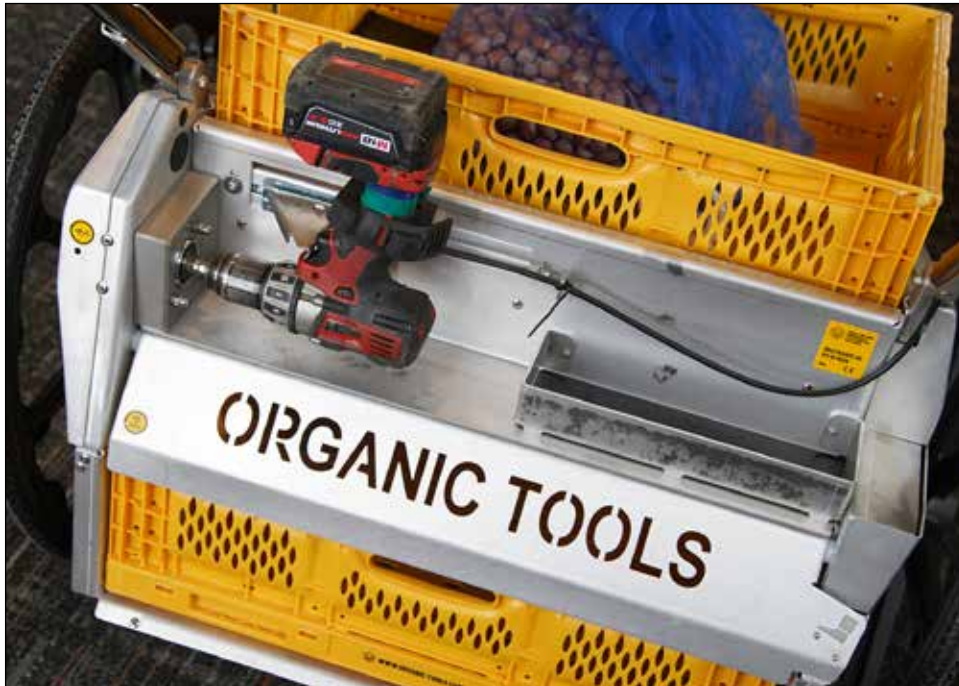
This hazelnut harvester can be powered by a drill attachment or e-bike battery.
