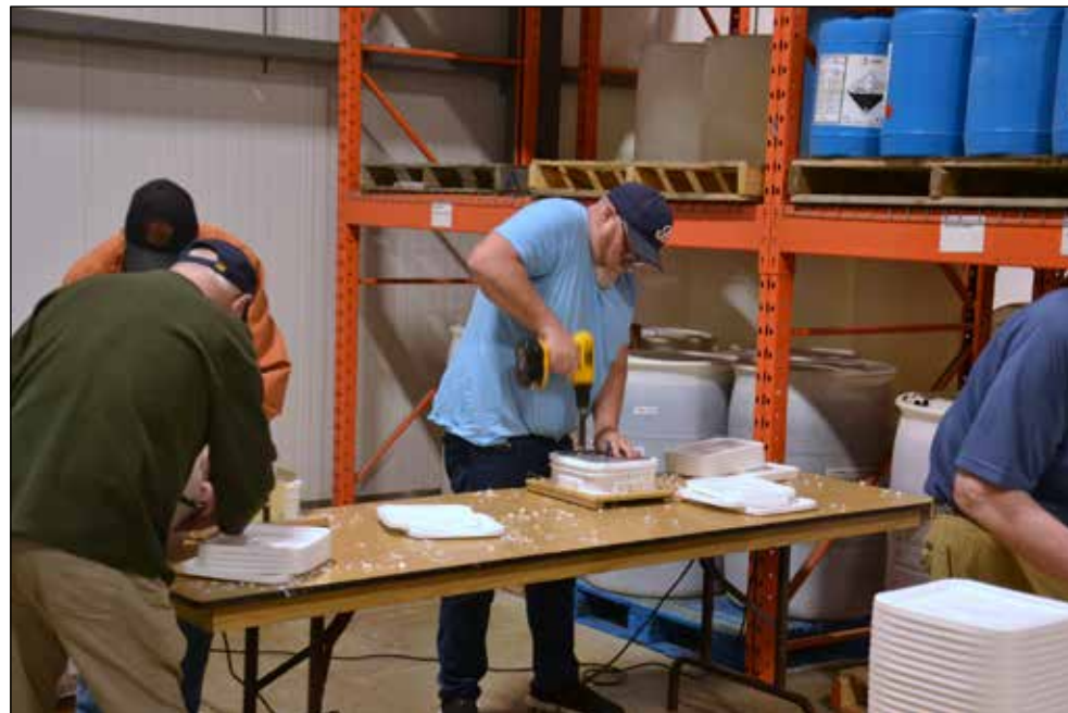
Volunteers drill holes in the Aquabox lids where two ceramic water filters will be installed.
