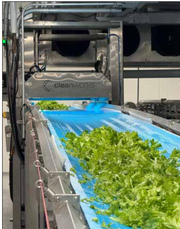
Cleanworks Corp.’s patented process reduces pathogens – E coli, salmonella, listeria and such – 99 to 99.9 per cent, making food safer; it also drastically reduces mold and mildew, meaning it lasts longer, too.
